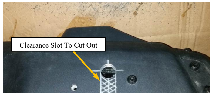
EXAMPLE OF HOW TO CUT CLEARANCE SLOTS. PICTURES MAY NOT LOOK LIKE YOUR BUMPER.
